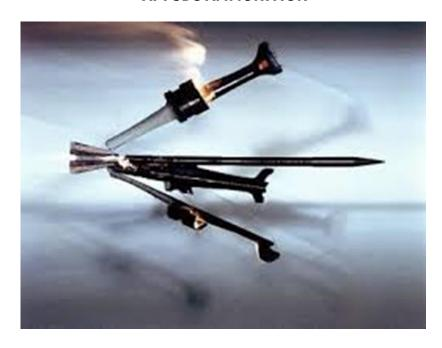
SABOT AND PENETRATOR SEPARATING BEYOND GUN BARREL
